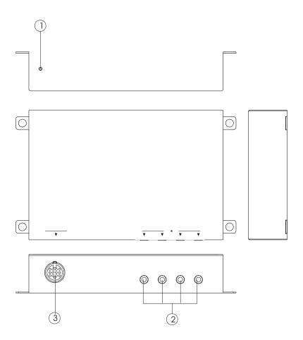
This unit can't be used separately and it must be used with other special system with the 13 -pin cable. The unit is connected to another system through the 13-pin din socket (3). And the unit can receive TV signal through the antenna input jack (2).
